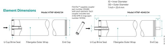
FilmTec<sup>™</sup> coupler part number 89048 is ordered separately for each element. Each coupler includes two 2-210 EPR O-rings (part number 89255).
