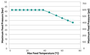
Figure 1: Maximum allowed temperature and pressure for FilmTec<sup>™</sup> HTNF-8040/34 and FilmTec<sup>™</sup> HTNF-4040/34
