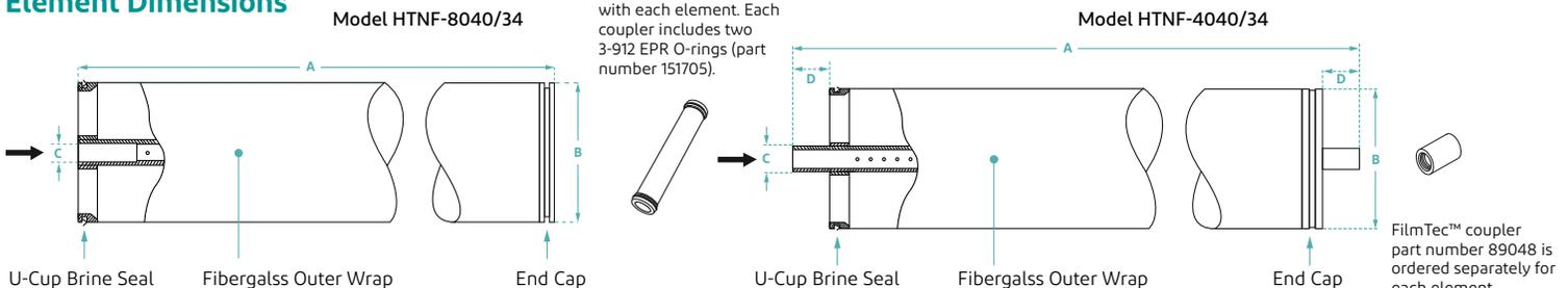
FilmTec™ supplies coupler part number 255289 with each element. Each coupler includes two 3-912 EPR O-rings (part number 151705).
