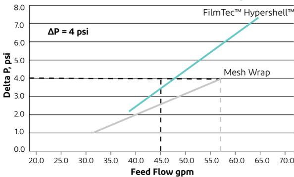
**Figure 1: Feed Flow vs Pressure Drop for Mesh Wrap and FilmTec™ Hypershell™ Elements.**
